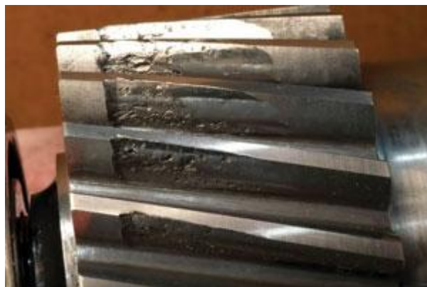
Severe misalignment can cause macropitting on helical pinion gears.
